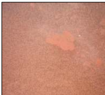
Fig 2: DOM binds with Fe(III) forming large particles removed by sedimentation or flotation.
